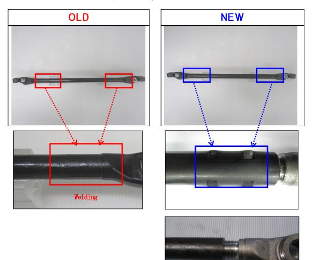
Sleeve(Tube) is joined to Socket tightly with screws and punches.
