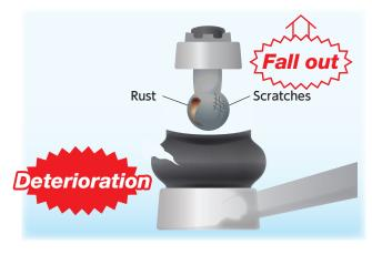
If the dust cover is broken, the ball stud is getting rusty and worn out. It is getting loose and might be coming out in the worst case.
