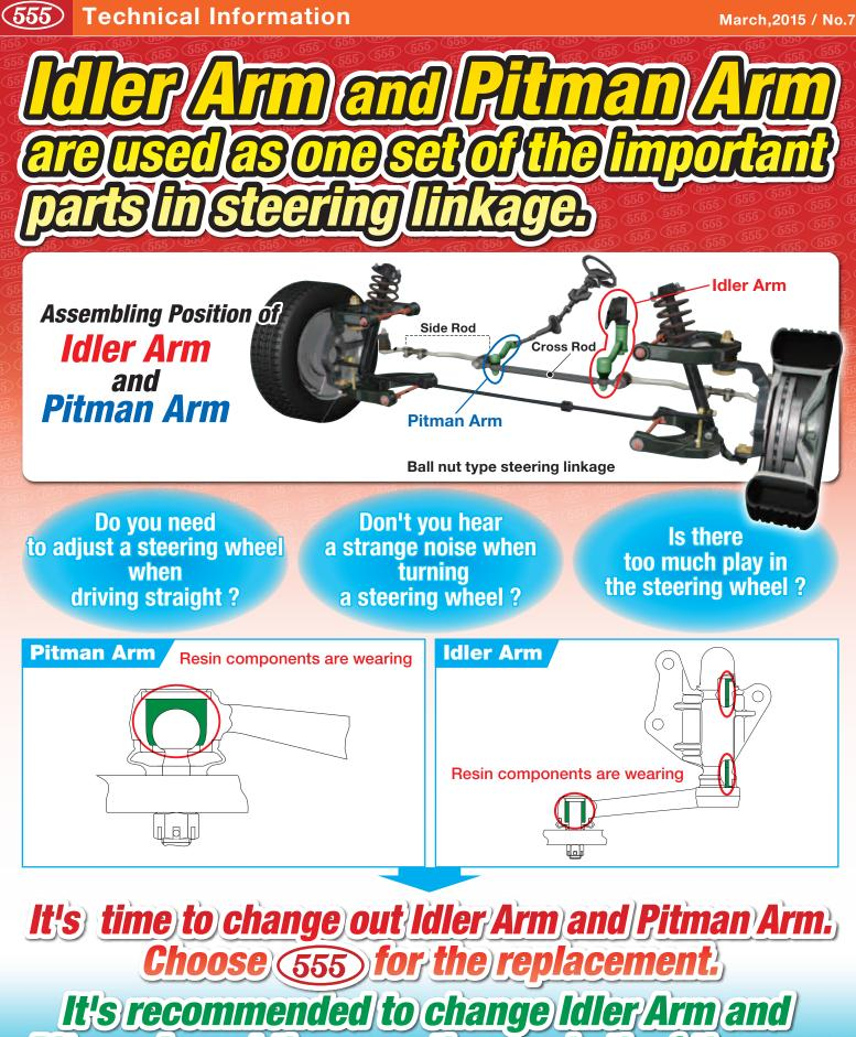
It's recommended to change Idler/Arm and Pitman/Arm at the same time, as both of them are worn away together by heavy friction motions.
